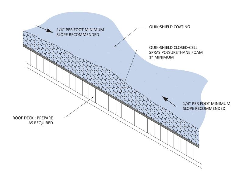
FLAT ROOF SLOPED WITH FOAM
