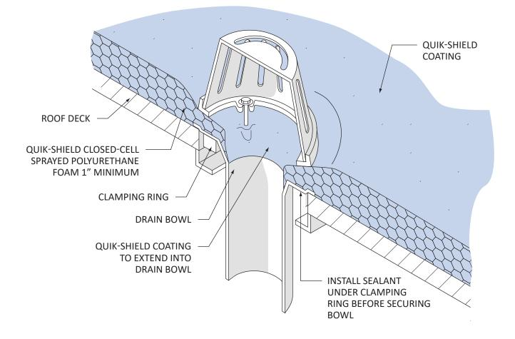
**ROOF DRAIN WITH MECHANICAL FASTENER**
