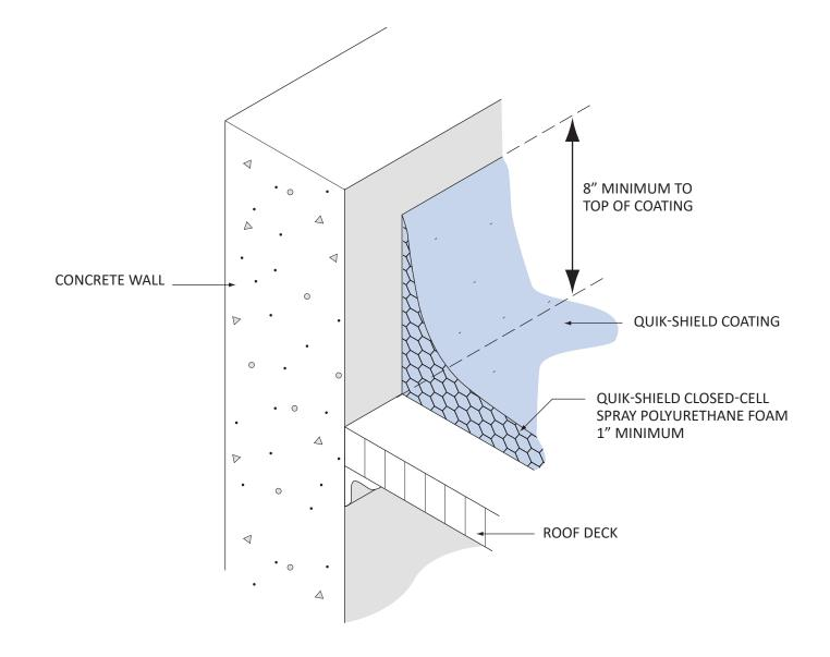
NOTE: THIS DETAIL TO BE USED ONLY WHEN DECK IS SUPPORTED BY THE WALL
