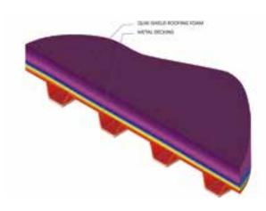
1" or more of QUIK-SHIELD® spray foam significantly reduces heat transfer through studs, fasteners, and roof deck gaps
