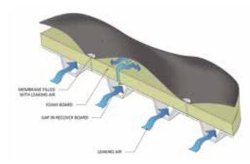
Fasteners and seams allow air to leak beneath the membrane. The wind pressure can cause fluttering of the membrane and, potentially, roof blow off
