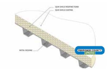
QUIK-SHIELD® spray foam on a metal deck maxed out the Miami-Dade wind uplift test at over 500 mph.
