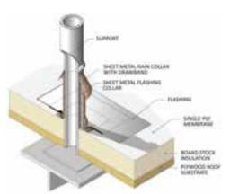
Traditional roofing solutions do not form a monolithic seal on penetrations and therefore have high leak potential
