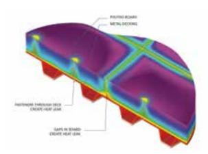
Fasteners and seams on Single-Ply roofs allow heat to transfer, wasting energy and money
