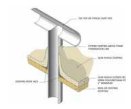
QUIK-SHIELD® spray foam is self-flashing and forms a seamless seal on roof deck penetrations
